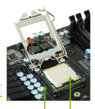
Align notches with notches on the CPU
