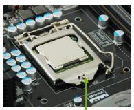
Load plate tip under screw cap
