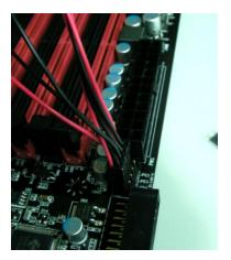
It doesn't matter which end of the PCIE Cable goes onto the Motherboard. Please be reminded to do this when PC is not running.
