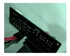
The Red wires should be occupying the pins on the top row.
