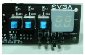
From Right to Left, PCIE Slots 1,2,3. When Jumper is in top position, PCIE slot is enabled. When in bottom position PCIE slot is disabled. Above shows example of PCIE slot 2 disabled while the rest are enabled.
