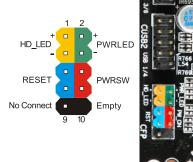
Note: Some system cases do not have all four cables. Be sure to match the name on the connectors to the corresponding pins.
