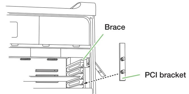
5. Remove the port access covers **2** from the slots in which you plan to install the card or remove an existing graphics card if present (Figure 2).
